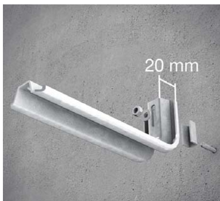
2 | Wall mounting with bracket KSLW To install the bracket KSLW use a dowel such as e.g. SD 8/30*. The spacer KSL-SP must be positioned before the dowel.
