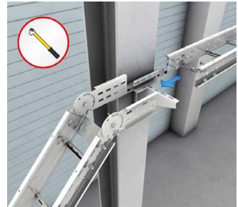
21 | Vertical wide-span couplers Insert a connecting cable ladder into the couplers (WPVV) and attach it with four bolts per side rail.
