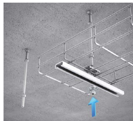
6 | Central suspension for wire mesh cable tray of up to 300 mm width Connect the central hanger GBAG 20/30 to the dowel using a hexagonal connector VM M8*. Mount the connector GV 30 as well as the profile rails with the wire-mesh cable tray inbetween both.
