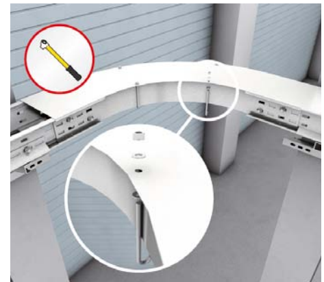
27 | Cover clamps Attach covers to wide-span cable ladder fittings (WPBD, WPAD or WPKD) with cover clamps (WPFDK) at every hole.
