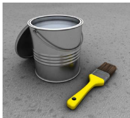
32 | Galvanised After the deburring, all cut areas must be galvanised with cold zinc paint (KZF) or cold zinc spray (KZS) on site.
