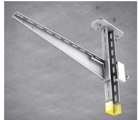
6 | Ceiling mounting with heavy bracket support KDU 60 To install KDU 60 use two dowels such as e.g. SD 10/10*. Then attach the bracket KW using head screw set KLS 10x20*. If the bracket is longer than 500 mm, screw the support piece KHUSS together with the bracket. The protection cap SU 60* is fitted to the bracket bottom, if needed.
