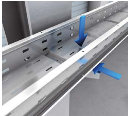
2 | Flange mounting clamp Place wide-span cable tray in position and push against screwed flange mounting clamp (WPHS). Make sure the wide-span cable tray is in the correct position!
