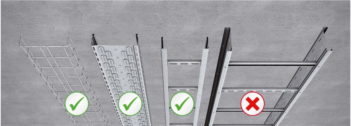
Installation instruction for support systems of wire-mesh cable trays, cable trays and cable ladders attached directly to concrete.
