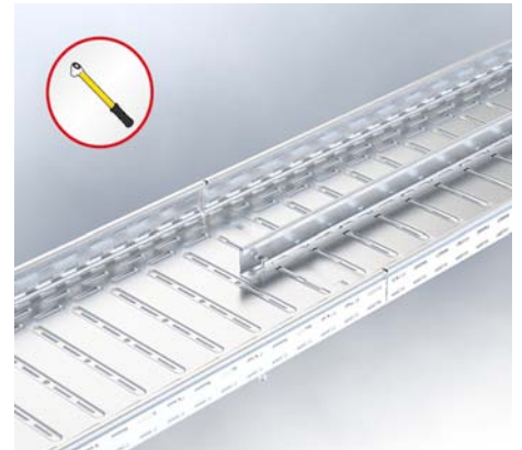
30 | Barrier strip Screw barrier strip in three places (approx. 100 mm from both barrier strip ends as well as in the middle).
