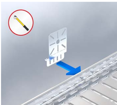
31 | Assembly plate Screw the assembly plate (MP-RG) for electric components to the side rail of the cable tray in two places.
