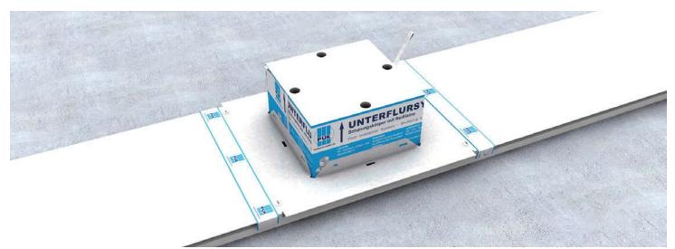
Open, two- respectively three compartment cable duct UKR in the nominal widths B = 300, 400 and 500 mm, made of steel sheet with length L of 3000 mm. In heights of 35, 60, 85 and 110 mm. Loading capacity up to 0,75 kN. Consisting of a bottom piece with a barrier strip and a separate top piece.
