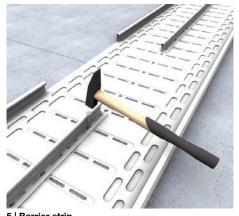
**5 | Barrier strip** Always fasten barrier strips UKTR symmetrically to the rough concrete using plugs once per metre.
