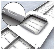
**13 | Assembly cover** The assembly covers UKDA are levelled dead centre in duct course and mounted to the duct using turning bolts. All conductive parts must be considered in the potential equalisation.
