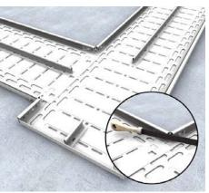
**9** | Final assembly of fitting components The barrier strips must be cut flush at the notches of the extensions and junctions. Trim the interfaces neatly and cold-galvanise.
