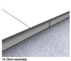
Mount duct bottom piece and dummy cover on parallel offset.
