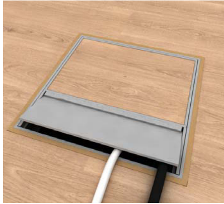
8 | Single outlet Insert rubber seal and cartridge cover, in case of dry maintenance floors install cartridge unit with cable outlet. The unit must be integrated in the potential equalization of the system.
