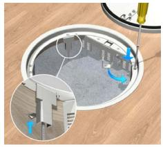
**3 | Claw fastener**Fit the provided claw fastener with the appropriate screws in the frame and tighten them.
