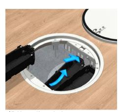
4 | Rubber seal/mounting box For the impact noise decoupling, the rubber seal is already sticked into the cartridge installation unit. Snap in the mounting box(es) as deeply as possible. In case of using a connector plug with H = 35 mm, the necessary installation depth is 85 mm.
