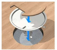
1 | Cartridge installation unit Insert the cartridge installation unit (UEKDD R E) which is usable for up to three mounting boxes in the floor opening.
