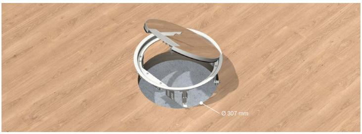
Cartridge installation units with a protective floor covering frame made out of stainless steel, round, with an outside diameter = 330 mm, for hollow space or false floors, with a clamping range from 40 to 80 mm. Usable for floor coverings with a thickness of 12 mm.
