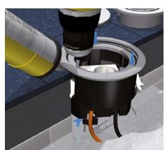
4 | Attach the frame and insert the strain relief
