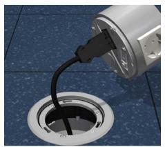
**10 | Connecting cables** Insert the plug of the 3-pole connecting cable in the snap-in of the floor plate.
