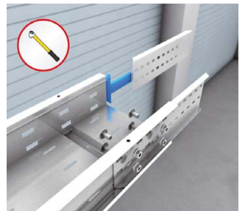
6 | Wide-span coupler Push wide-span coupler (WPV) into the side rail of the wide-span cable tray and screw four times per side rail with clamping screw (KLS 10x20).
