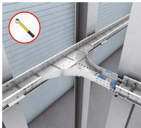
23 | Branch-piece Insert connecting tray with connection plate (VB) into extension branch-piece (WPRAA) and screw four times per side rail.
