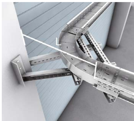
5 | Heavy corner installation EBW Heavy corner installation (EBW) for horizontal 90-degree turnarounds with side rail support (WPHS-K) are to be plugged to concrete support. L = width of wide-span cable tray + 560 mm
