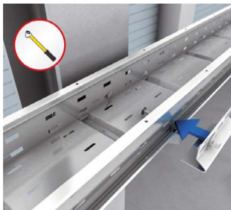
5 | Flange mounting clamp Push flange mounting clamp (WPHS) onto the bracket and screw together with the wide-span cable tray and the bracket.
