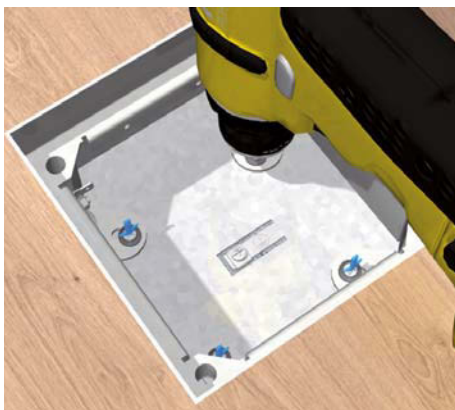
4 | Fixation Insert the frame and mount the four levelling legs onto the bottom of the hollow floor box with nail plugs.
