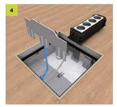
Lock-in leads Mount both lock-in leads with two screws each on the side of the frame. Create grounding connection between levelling device and floor box. When using a coupler plug H = 35 mm, comply with the minimum installation depth Hmin = 95 mm.
