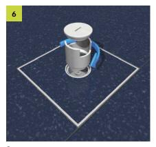
Stone cover For wet maintenance floor covers such as stone covers, only a tube cartridge unit may be used. However, the floor cover depth must be considered. Insert the replaceable cartridge into the frame. The tube can be screwed. Observe the potential equalization.
