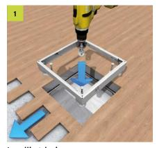
Levelling device For parquet or stone floors insert the levelling device into the floor opening. Fasten the four levelling bases with nail plugs.
