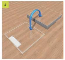
**Parquet cover** For damp maintenance floors such as parquet covers, use a dummy cartridge unit or a cable outlet cartridge unit. However, the floor cover depth must be considered. Insert the replaceable cartridge into the frame. Observe the potential equalization.
